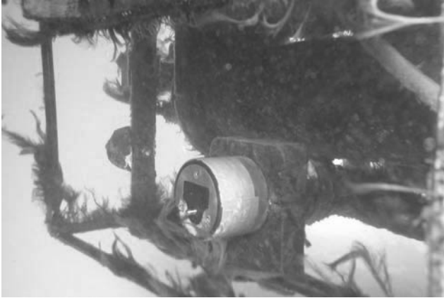
Fig. 4. Underwater photograph of WET Labs fluorometer, after 5 months in the water., Anti-biofouling copper tape has kept algal growth from affecting the optical window even though it was deployed without a shutter. Photo by Steve Karpiak, MER.
